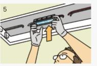
Replace the removed ballast with the LED SMPS and connect the wires.
