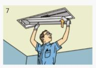
Check if the LED SMPS has been connected correctly and reassemble the lamp fixture.
