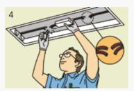
Make sure the power is shut off to avoid electric shock, then cut the wires connected to the ballast.
