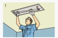
Detach existing fluorescent lamp. (Switch off the power before operation)
